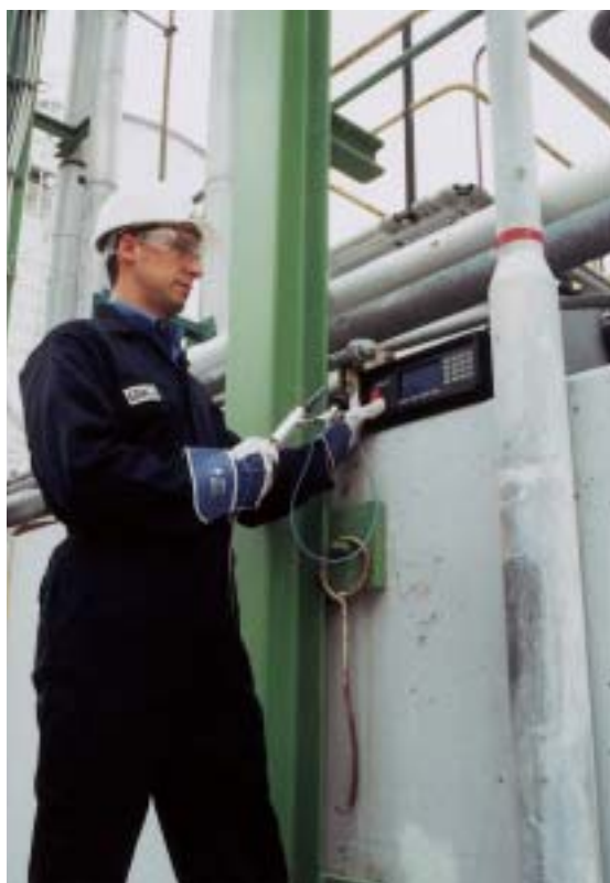
On-Site Breakthrough Measurement by a GRACE Davison Engineer
